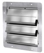
The BD-320 is a vertical mount backdraft damper designed to allow horizontal airflow and prevent reverse airflow. The dampers are opened by air pressure differential and closed by gravity. The damper features a galvanized steel frame with a flange on the discharge side and aluminum blades.
